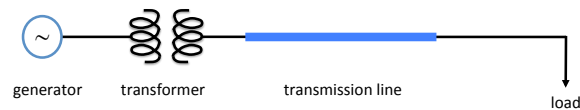
Figure 4.3: One-line diagram of a generator supplying a load through a transformer and a transmission line.
